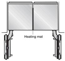
If the appliances are installed directly next to each other (without a partition), they will need to be attached together. A heating mat must also be installed. This will help avoid condensation and prevent damage.
